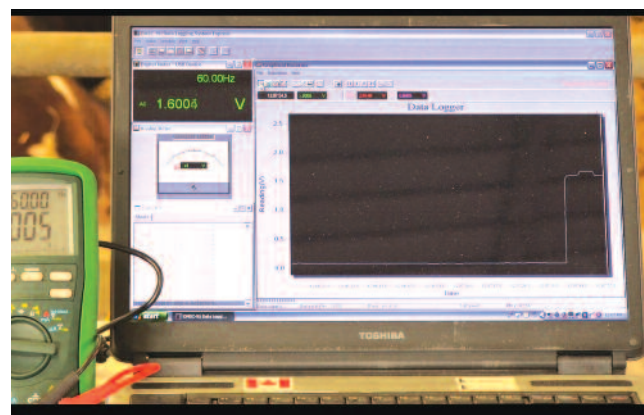
Equipment used to determine causes of ground current on a farm.
