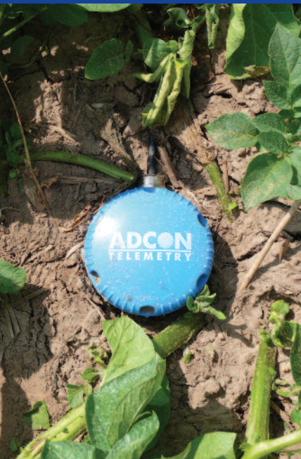
This soil moisture probe stays in the soil and determines moisture levels at 10cm, 20cm and 30cm.
