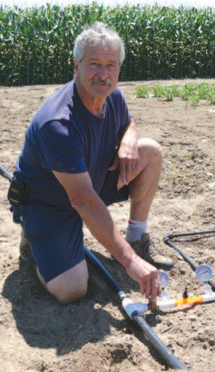
Peter White of the Simcoe research station kneels next to a pressure sensor of the subsurface drip irrigation system being used to irrigate corn.
