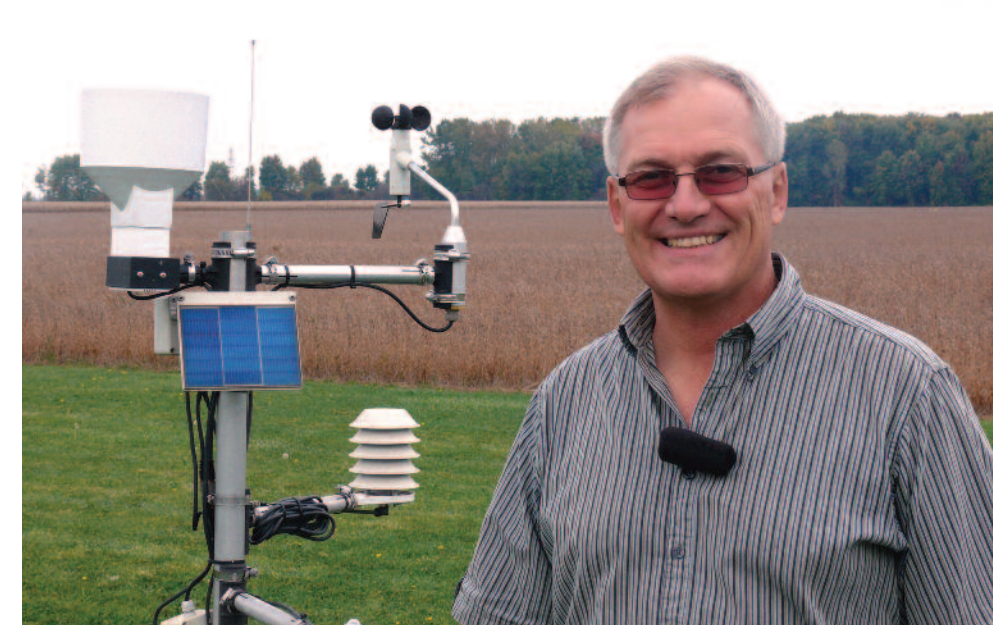
Ian Nichols of Win Weather Innovations stands next to a weather station that monitors variables such as temperature, relative humidity and rainfall.
